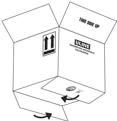
1. Fold flaps on bottom of carton so that they meet. Manufacturer's certification must be visible on the outside of the carton. (See Figure 1)
