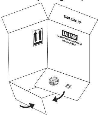
3. Seal bottom of carton with three parallel strips of 2" wide (2.6 mil) polypropylene tape (Uline Model # S-14564). The tape must overlap 0.5" side to side and extend 3" over each end of the carton. (See Figure 2)
