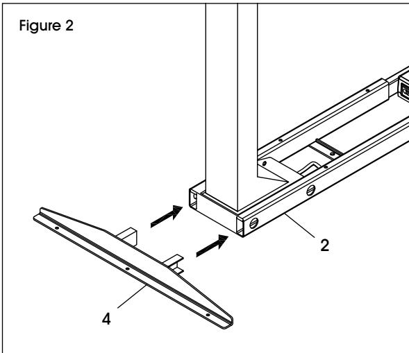
4. Insert two M6 x 33 mm machine screws (9) into holes on end of adjustable frame to connect adjustable frame with lifting columns and top support bracket. Lightly tighten using 5 mm hex wrench. Then lightly tighten two pre-installed M6 x 33 mm machine screws (9) to secure lifting column. Repeat this step on the opposite side. (See Figure 3)
