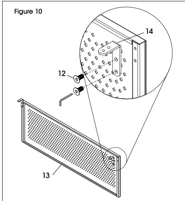
13. Position metal modesty panel (13) centered between frame on back of desktop. Attach modesty panel brackets (14) using two M5 x 20 mm wood screws (11) per bracket. (See Figure 11)
