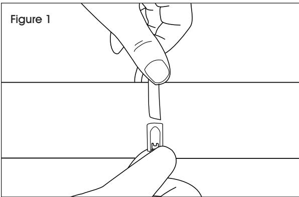
2. Insert end of tie into mouth of machine. (See Figure 2)
