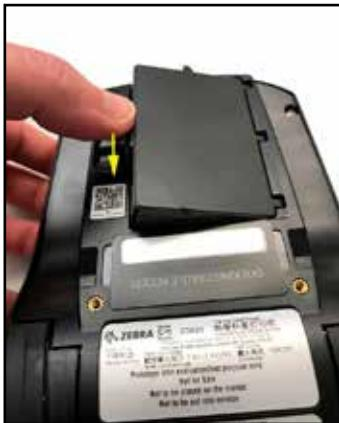
4. Rock the battery into the compartment as shown until it locks in place.
