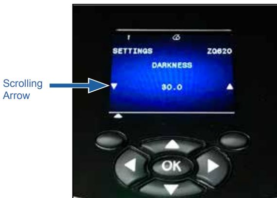
Some parameter settings like the Darkness setting above have a scroll option to view multiple setting choices. This option is identifiable by the presence of up and down scrolling arrows located on either side of the display (see Figure 18). Press the up and down arrows on the keypad to scroll through a menu's options. In some cases, further actions will appear on the right side of the status screen (see arrow in Figure 19). Press the right soft key to initiate said action.
