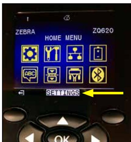
The user can scroll between icons using the four-way arrow buttons. When an icon is highlighted (i.e. Settings), its text description will be displayed in the middle of the navigation bar (see arrow in Figure 17), and can be selected by pressing the "OK" button. This will take the user to the first screen (i.e Darkness) under that parameter, which gives the user status information specific to that option (see Figure 18). In order to navigate to the next screen, click on the right arrow button.
