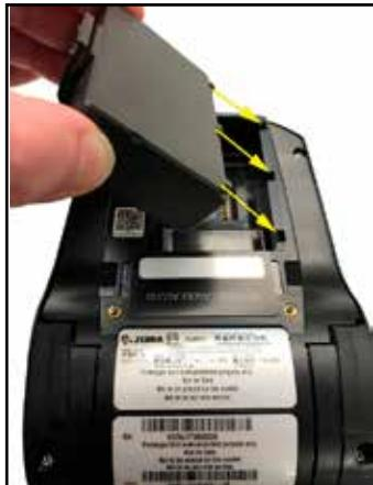
3. Insert the battery into the printer as shown. (It is not possible to insert the pack in the incorrect orientation.)
