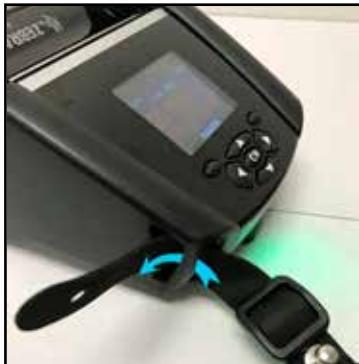
1. Insert the end of the shoulder strap behind the post on the front side of the printer and loop it around the post.
