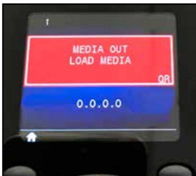
The user can respond to actions by pressing one of the soft keys to indicate that an action has been taken to address the alert in question. Once the condition causing the alert has been addressed (i.e. loading media), the alert message will be cleared. (See Appendix G for a complete list of alerts for the ZQ6 printers.)
