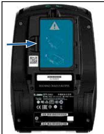
3. Rotate the pack away from the battery well. Lift the battery up and out of the printer.
