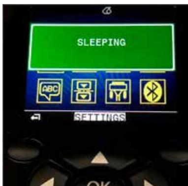
When the printer is in sleep mode, the green LED ring around the power button will pulse approximately once every three seconds. Pressing any button on the printer will wake the printer from sleep mode. Other power management features of the ZQ6 printers include “wake on Bluetooth” and “wake on WiFi” whereby the printer exits sleep mode due to data exchanged via Bluetooth 4.1 or a network message received over WiFi. The printer will not enter sleep mode when docked in an Ethernet cradle.
