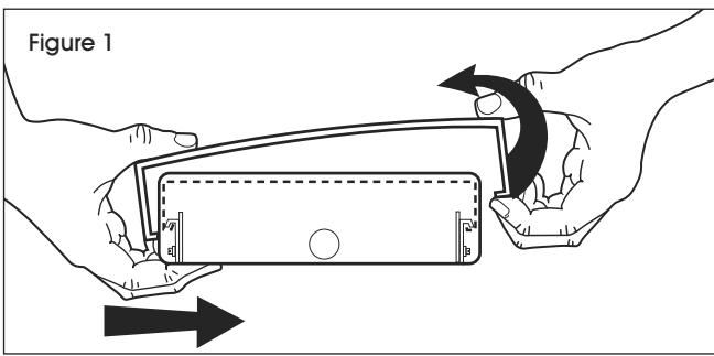
2. Remove wireway cover from housing by squeezing wireway cover to disengage from retaining slots.
