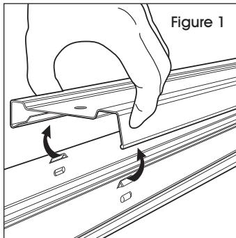
2. Place track assemblies into slots in the end of channel.
