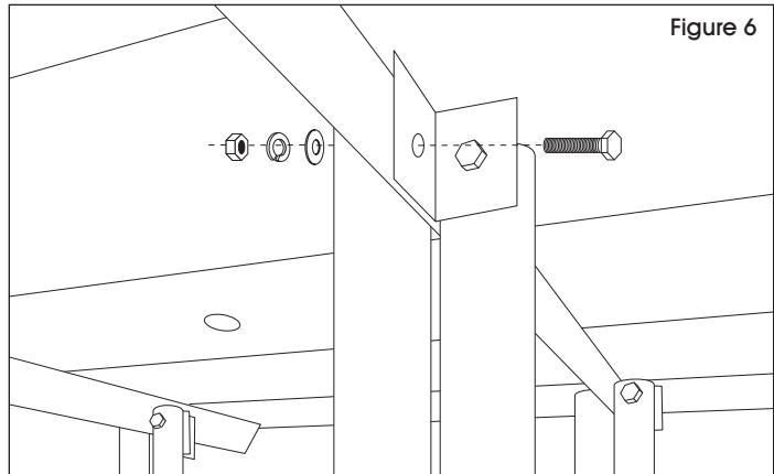
8. Attach the bottoms of the legs to the X-Brace using 2½" hex bolts. Secure using a lock washer and hex nut.
