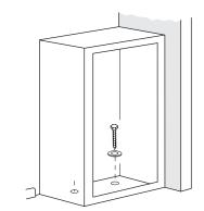
5. Secure the safe with fasteners and replace carpeting.
