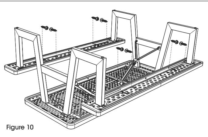
14. While one person holds the table legs upright, insert four screws through the holes in the bench channels and into the bench as shown to keep the sliding end caps under the glide rails. (See Figure 10)
