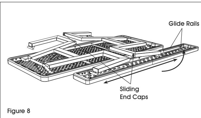
10. Attach two sliding end caps to the tube on the other table leg, and lift the bench seat upward until the sliding end caps rest inside the underside of the bench. Position the bench so all four sliding end caps are under the glide rail. (See Figure 8)
