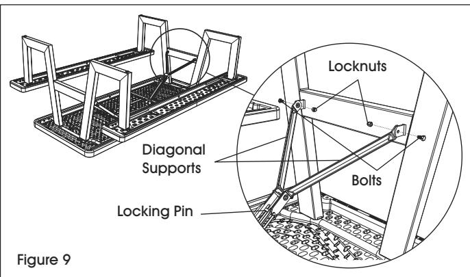
12. Lift one leg assembly upright and hold it in place. A second person will rotate the diagonal supports of the leg brace assembly until the locking pin snaps into the notches located at the end of the diagonal supports. Connect the ends of the diagonal supports to the leg assembly using two bolts and two locknuts. (See Figure 9)
