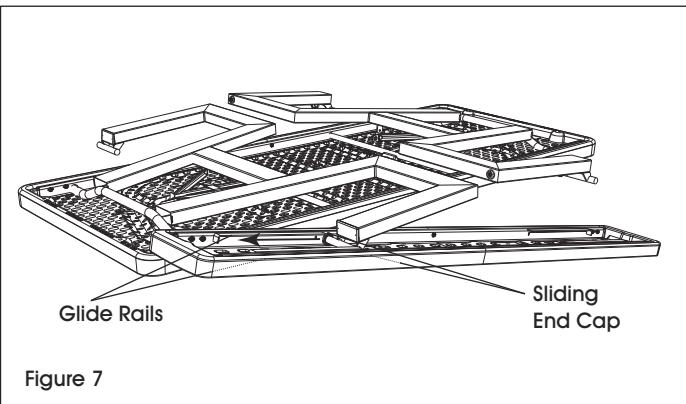
9. Place a bench seat underneath one of the legs and slide the sliding end caps under the glide rails of the bench seat. (See Figure 7)
