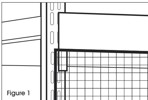
1. Align the pallet rack netting with the center of the upright and the bottom of the shelf beam. (See Figure 1)
