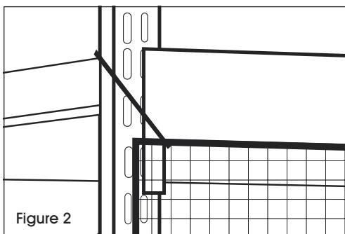
2. Secure the corner of the pallet rack netting with a cable tie. (See Figure 2)
