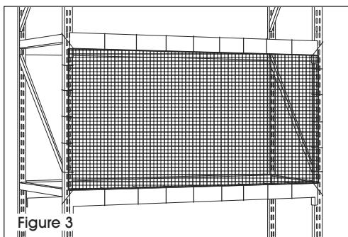
3. Secure the rest of the pallet rack netting with a cable tie every 12" on each side. (See Figure 3)
