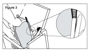
Once the cartridge is 3-4 inches below top of tracks, remove the yellow ribbon and cardboard. (See Figures 4-5)
