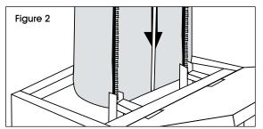
Push down and forward (keeping the cartridge at a 90° angle), ensuring all blue clips enter the track. Use both hands if necessary. (See Figure 3)
