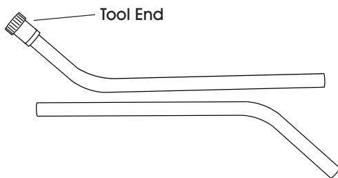
2. Align the wand ends together. Attach by pushing together until you hear a click when the push button locking pin is inserted through the hole.
