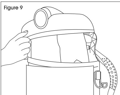
4. Separate lid from paper bag insert and dispose of paper bag. (See Figure 10)
