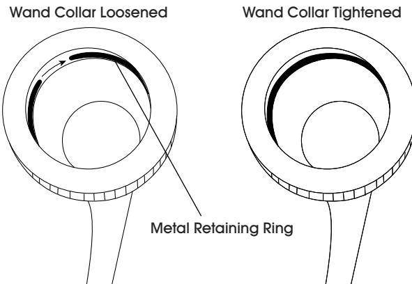
5. Insert the floor tool head and tighten the collar. (See Figure 6)
