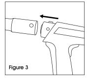
Assemble the combustor on the end of the extension and confirm it is locked in place by the #31 button. (See Figure 2)
