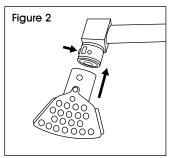
4. If any of the O-rings are damaged, replace them before using the tool.
