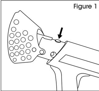
2. Assemble the combustor on the end of the extension and confirm it is locked in place by the #31 button. (See Figure 2)
